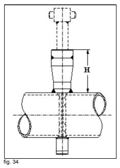
For Itabar®-sensors type IBFD-HT the standard H-dimension is 168 mm.
