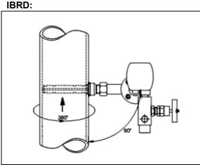
fig. 3: IBRD installed in a vertical pipe
