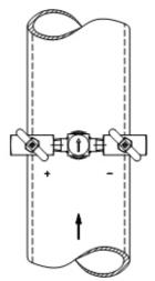
fig. 1+2: Arrangement of pressure tapping in horizontal and vertical pipes
