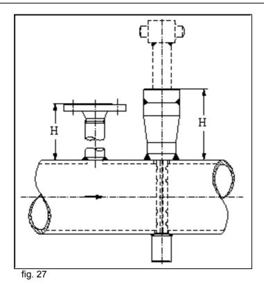
For Itabar-Flow-Sensors type IBFD the following standard H-Dimensions are available:
