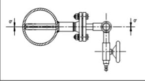
fig. 15: IBFD-25...-K7-A18 in a horizontal pipe
