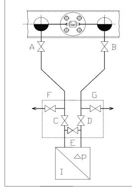
fig. 37 Sensor with condensate vessels K1
