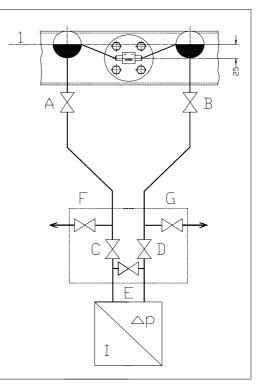
fig. 38 Sensor with condensate vessels K1
