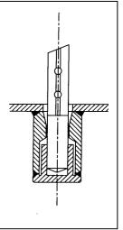
fig. 33: End support IBFD-HT, two-part welding construction
