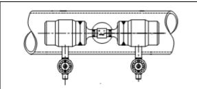
fig. 11: IBRD installed in a horizontal pipe
