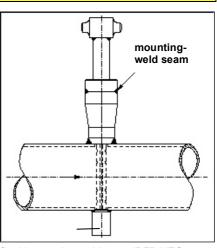
fig. 36 mounting weld seam IBFD-HTG
