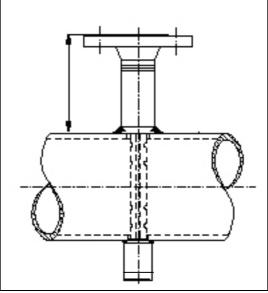
fig. 32: H-dimension for IBFD-HT-sensor
