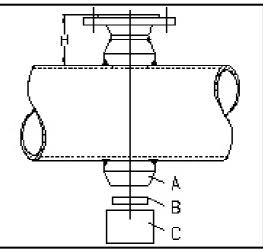
fig. 30 mounting parts sensor IBFD-21/26/36
