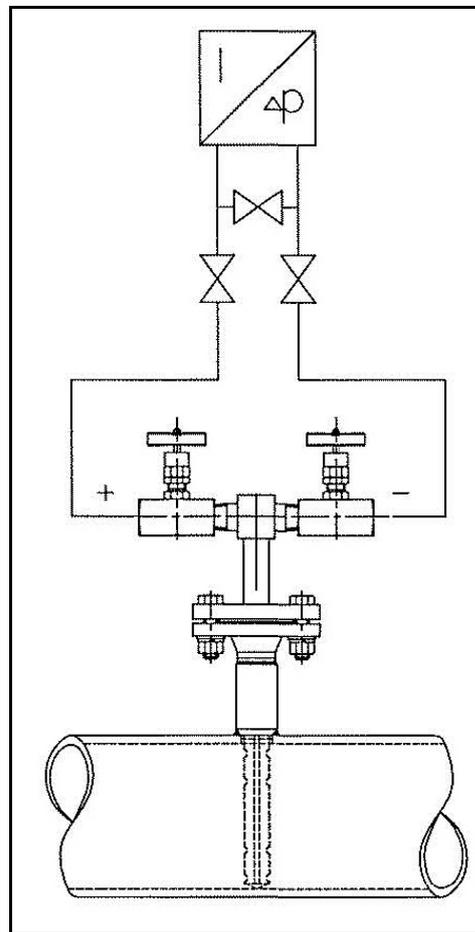
fig 15 Arrangement for dry gas and air flow measurement
