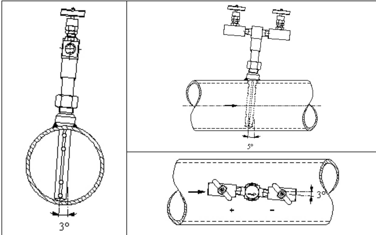
Fig 7 Allowable Misalignments.
