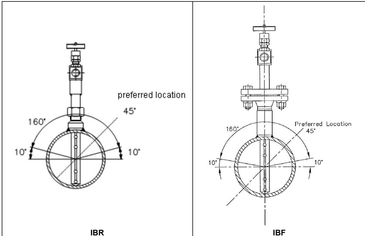
fig 6 Installation in horizontal pipe line for gases
