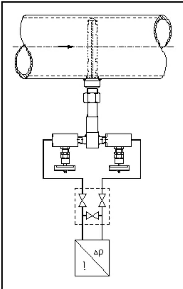
fig 14 Arrangement for liquid flow measurement
