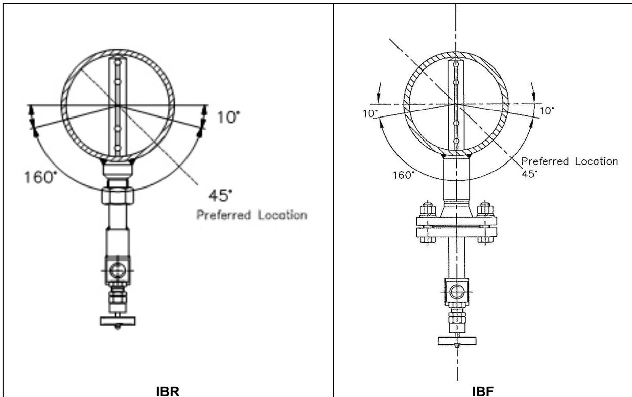
fig 5 Installation in horizontal pipe line for liquids
