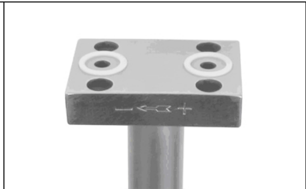
Fig. 34: Sensor head with flange plate to direct-mount a 3-way manifold. Limited use w/out pipe insulation, gases to pressure max = 63 bar (926 psig) and temp max = 200 °C (680°F) liquids to pressure max = 63 bar (926 psig) and temp max = 150°C (510°F)
