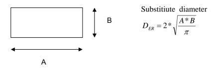
The sensor is always made for the longer side to better cover the flow profile.
