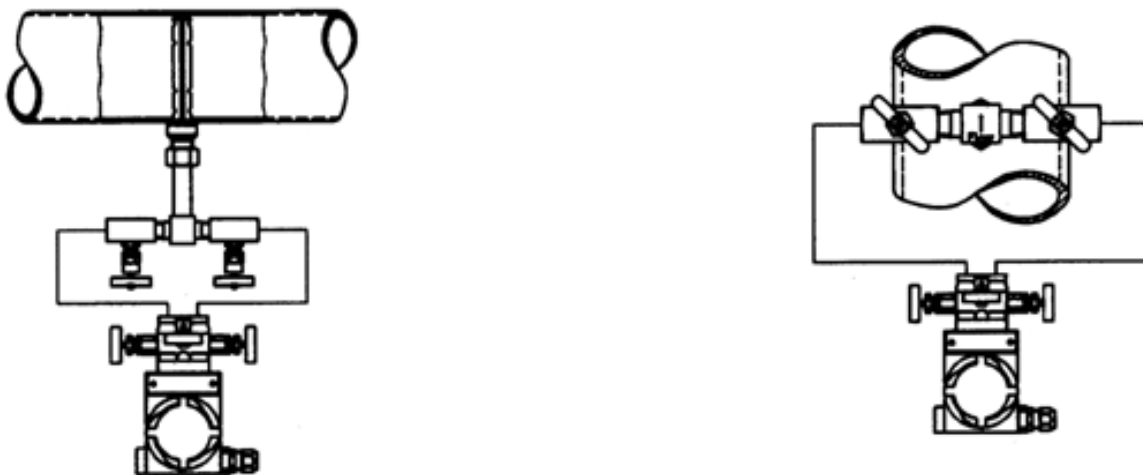
Fig. 45: Recommended sensor orientation for liquid measurement
