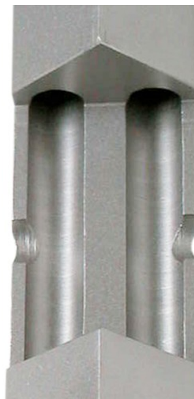
Fig. 8: Sensor profile of pitot tube model 35/36 in a cut-away view to illustrate the two pressure channels near the pressure ports..
