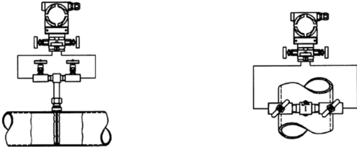
Fig. 44: Recommended orientation for measurement of gases
