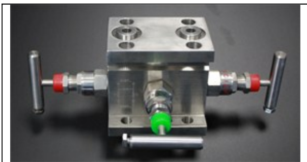
Fig. 22: 3-way-manifold PN 400 (5801 psi); 1.4401 (316SS) (A66)
