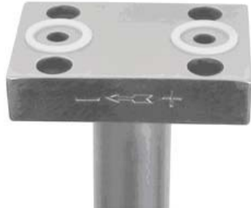
Fig. 34: Sensor head with flange plate acc. IEC61518 to direct-mount a 3-way manifold. Limited use w/out pipe insulation, gases to pressuremax = 63 bar (926 psig) and tempmax = 200 °C (680°F) liquids to pressuremax = 63 bar (926 psig) and tempmax = 150°C (510°F)
