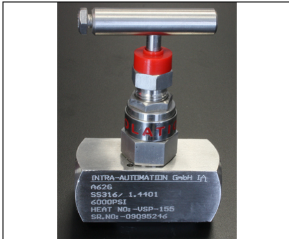
Fig. 21: Needle valve 1/2" NPT, PN400 (5801 psi; 1.4401 (316SS) (A62)
