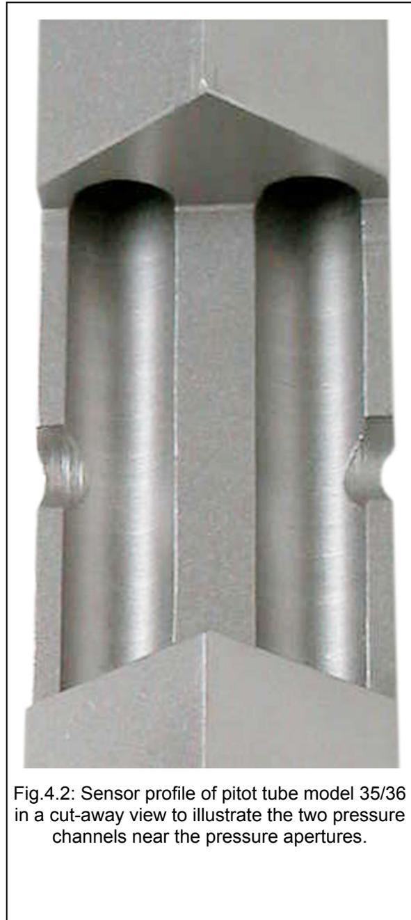
Fig.4.2: Sensor profile of pitot tube model 35/36 in a cut-away view to illustrate the two pressure channels near the pressure apertures.
