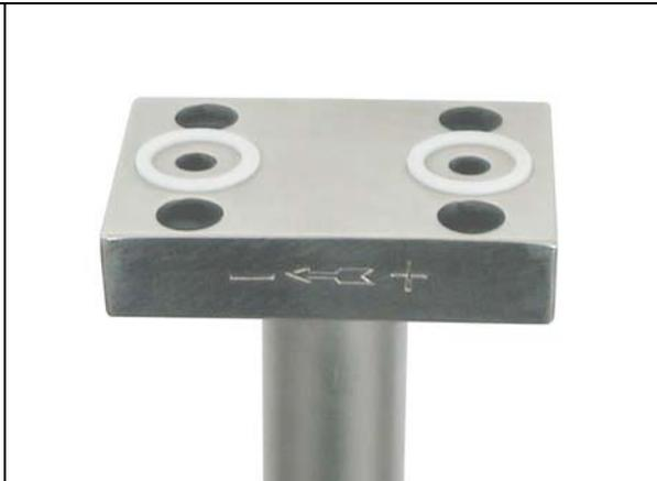
Fig. 7.2: Sensor head with flange plate to direct-mount a 3-way manifold. Limited use w/out pipe insulation, gase to pressure<sub>max</sub> = 63 bar (914 psig) and temp<sub>max</sub> = 200 °C (392°F), liquids to pressure<sub>max</sub> = 63 bar (914 psig) and temp<sub>max</sub> = 150°C (302°F)
