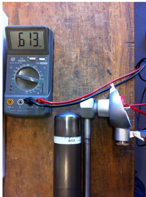
fig. 7: Ohmic signal at Full Scale
