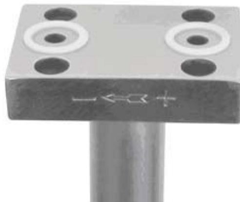
Fig. 34: Sensor head with flange plate acc. IEC61518 to direct-mount a 3-way manifold. Limited use w/out pipe insulation, gases to pressuremax = 63 bar (926 psig) and tempmax = 200 °C (680°F) liquids to pressuremax = 63 bar (926 psig) and tempmax = 150°C (510°F)
